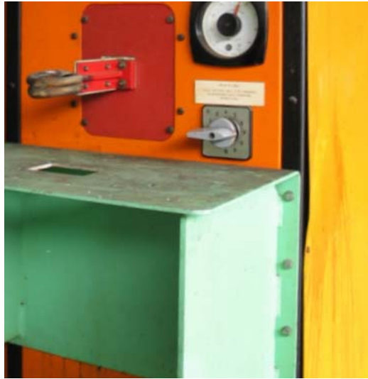
Figure 7 An induction heater with open coil - ready for overhaul.
