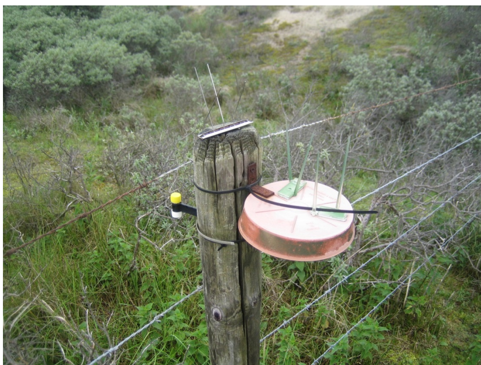
Figure 19: The Gradko sampler (left) and the housing of the ALPHA sampler (right) in the Meyendel bar.
