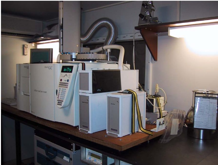
foto 1: Interieur mobiel laboratorium ML2, GC-MS Trace 2000 Thermo Finnigan Bron: RIVM
