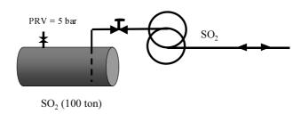
Figure 5 Sulphur dioxide tank
