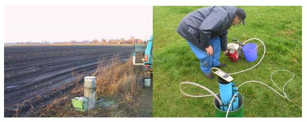
Figure 2.1 A multi-screen well next to a field (left) and the taking of samples (right).
