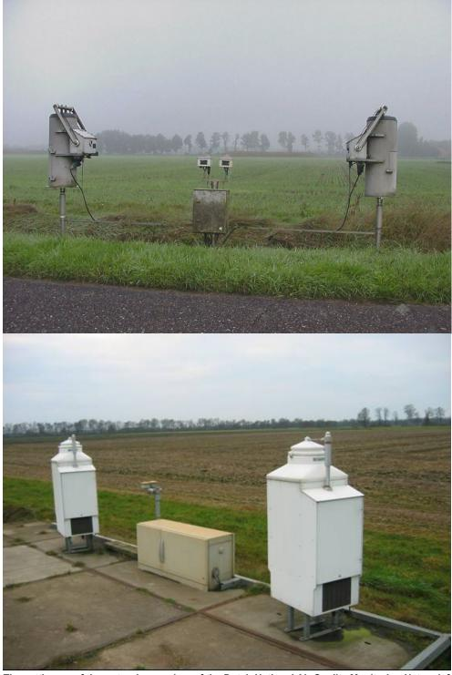
Figure 3 The setting up of the wet-only samplers of the Dutch National Air Quality Monitoring Network for Precipitation in Vredepeel (131) with the old samplers (top panel) and the new samplers (bottom panel)
