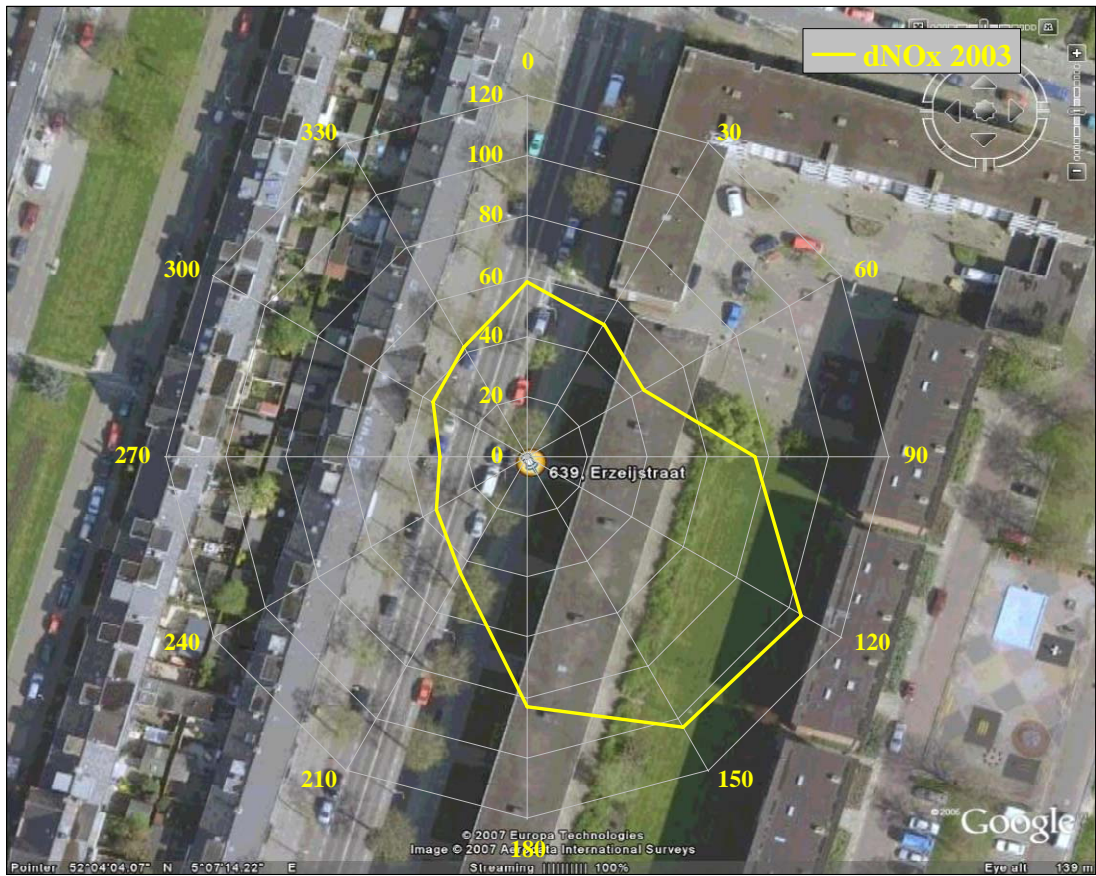
Figure 2 Wind rose of NO x concentration contributions in the Erzeijstraat. LML640 was used as the background location.
