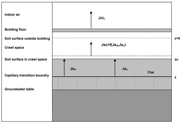
Figure 4-1: Transport fluxes of a contaminant from ground water through the unsaturated zone into the crawl space of a building a described by Waitz et al. (1996). The dotted line is the transition boundary
