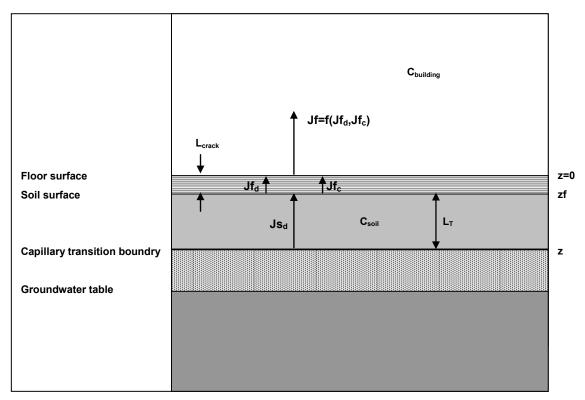
Figure 3-6 Transport fluxes from soil to the indoor air of a building with basement as described by Johnson and Ettinger (1991)
