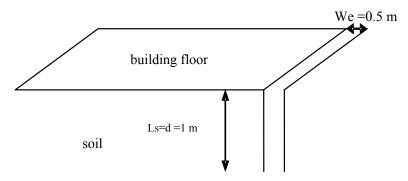
Figure 3-5 Schematic situation of the soil and building floor for convective air transport as described by Ferguson et al. (1995)
