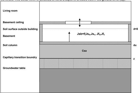
Figure 4-5: Transport fluxes of a contaminant from ground water through the unsaturated zone into the basement of a building
