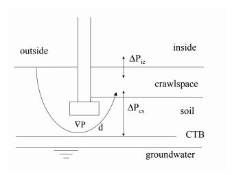
Figure 5-2 Pressure differences and airflow from soil to crawl space
