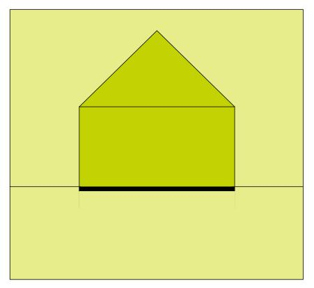
Figure 3-2 House with ground bearing slab (slab-on-grade)
