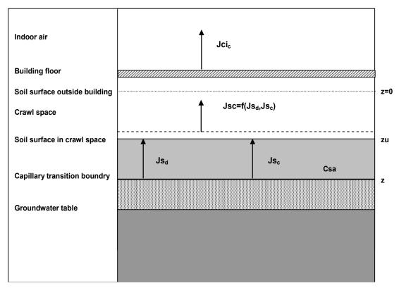
Figure 3-7 The transport fluxes of a contaminant from groundwater and the unsaturated zone into the crawl space of a building as described by Waitz et al. (1996). The total length of the unsaturated soil column Ls= z-zu. The dotted line is the transition boundary
