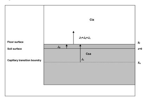
Figure 3-4 Transport fluxes from soil into a building with ground bearing slab as modelled by Ferguson et al. (1995)
