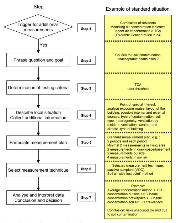
Figure 2-2: General approach of the risk assessment of volatile compounds in soil based on air measurements
