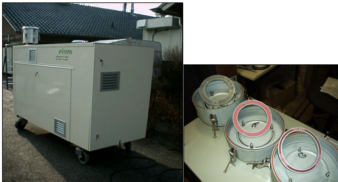
Figure 2.1 RAIAP PM collection device with the HVCI on top of a box with the pump to pull the air through the impactor (left panel) and the inside of the HVCI showing the pink PUF with collected PM (black) of the fine mode stage (right panel).
