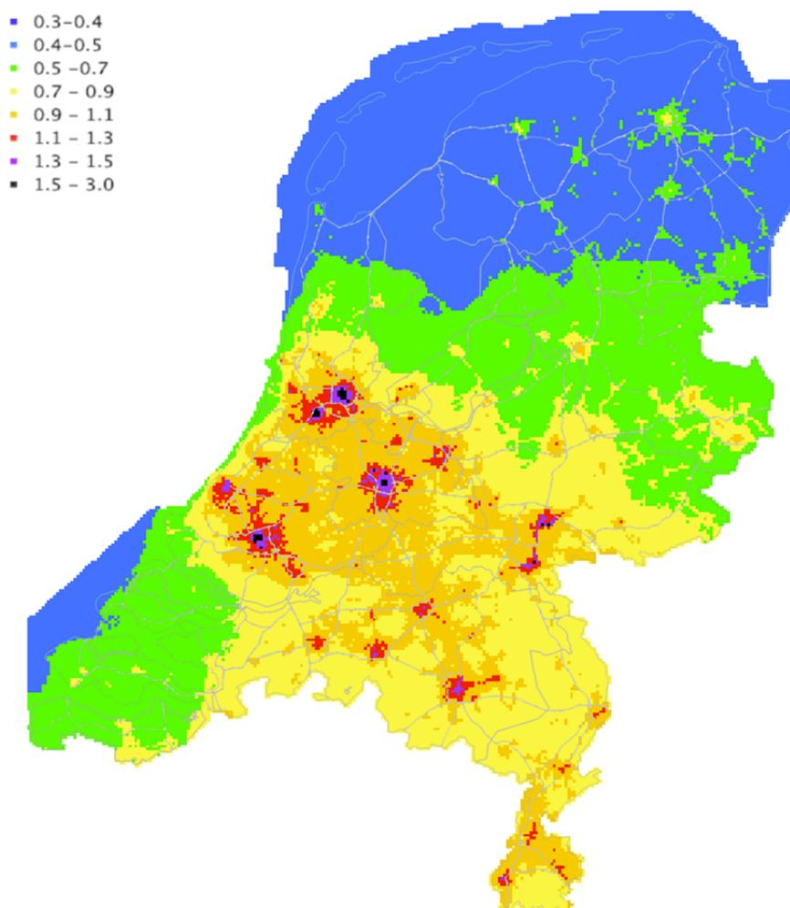
Figure 2 Uncalibrated calculated EC background concentrations for 2012. The scale, in  $\mu\text{g}/\text{m}^3$ , is shown on the left of the figure.
