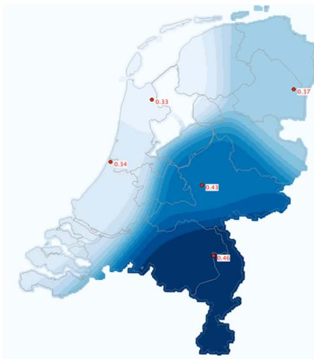
Figure 4 Interpolation of EC concentrations measured at rural locations for the whole area of the Netherlands.
