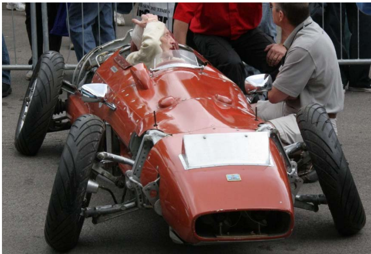
Figure 9 Wheel alignment has a major impact on the roadholding characteristics of the car and on tyre abrasion. Photo: Milliken MX1 Camber Car 1960 driven by Bill Milliken (Brian Snelson).
