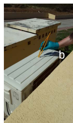
Figure 12 Dust sampling: wiping a Petri dish (a) and a 'historical wipe' (b).
