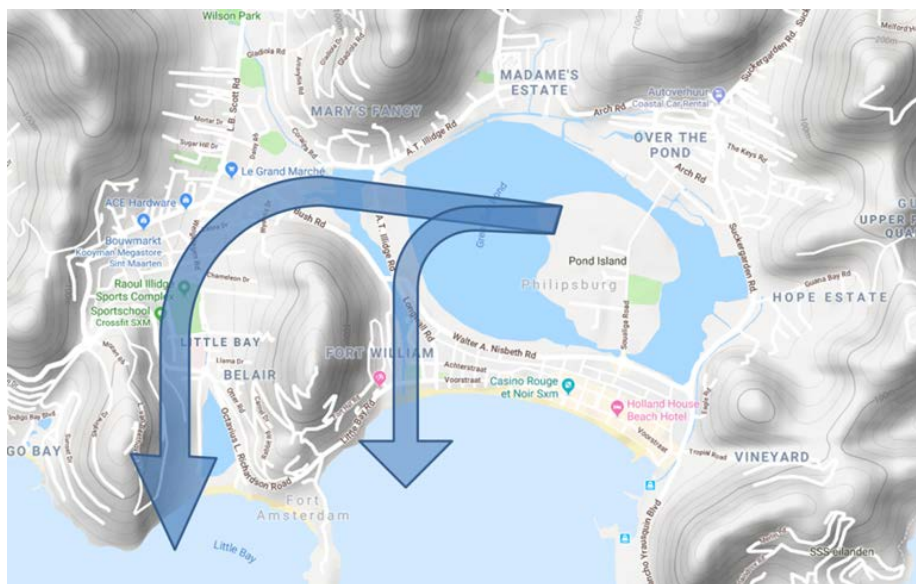
Figure 3 Local airflow under easterly wind conditions
