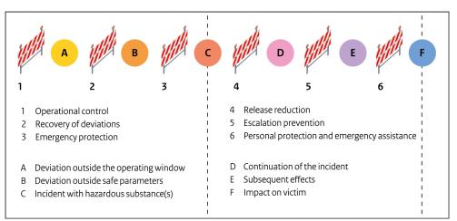
Figure 3.1. Lines of defence (represented by numbers) and the consequences of any failure (represented by letters) in the analysis model.
