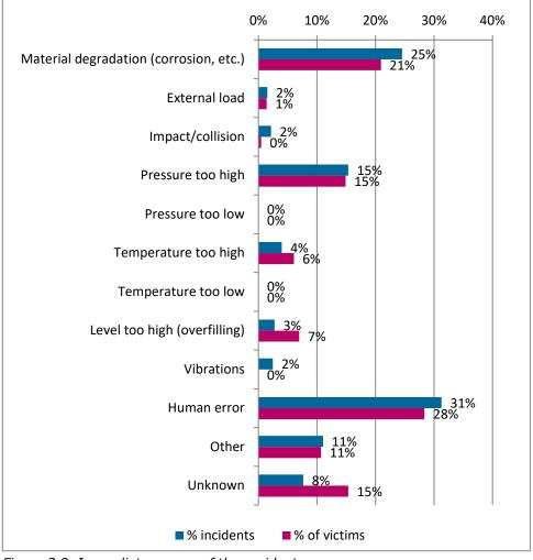
Figure 2.9. Immediate causes of the accident.
