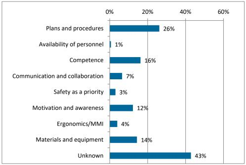
*Figure 3.11. Why do safety measures fail? Average incidence of management factors per safety measure failure.*
