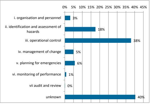
*Figure 3.12. Deficiencies in the SMS related to safety measure failures. The average incidence of deficiencies in the SMS per safety measure failure.*
