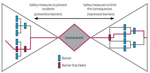
Figure A1.1. Storybuilder model with the incident path represented as a red line. This indicates the route of the incident scenario that occurred and the associated barrier failures.
