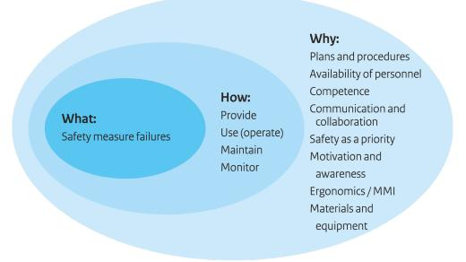
Figure A1.2. Structure for the underlying factors in the analysis model. The MDS management delivery system failures (why) precede the task failure (how), which precedes the barrier failure (what).
