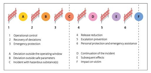
Figure A1.3. Summary of the Storybuilder MHC model. The lines of defence are represented by fences, the loss of control events by circles. The central event (C) is in the centre.
