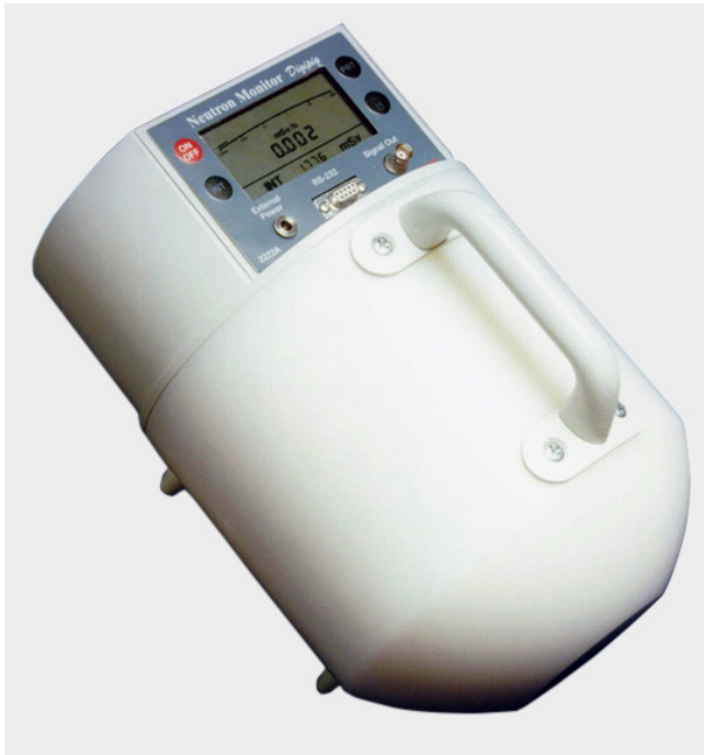
Figuur B1 Neutron Monitor Digipic, type 2222A (Southern Scientific)
