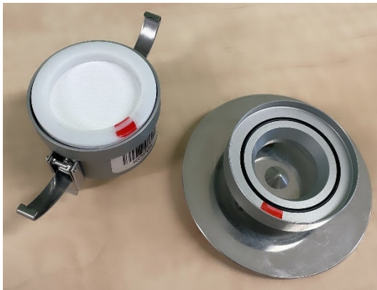
Photo 6 TSP filter head with quartz filter
