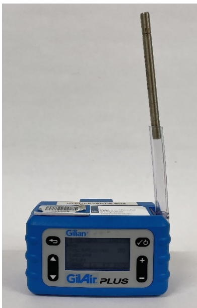
Photo 3 GilAir plus air pump, equipped with a thermal desorption tube
