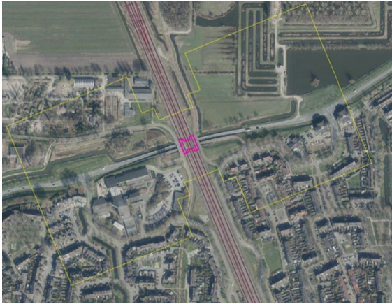
Figure 9.1 Example of determining an exclusion zone (yellow area) near a bridge (pink). The two red parallel lines indicate the tracks. The two distances to the left and right of the tracks are 50 and 100 metres (i.e. approximately 25 and 50 metres from the tracks).
