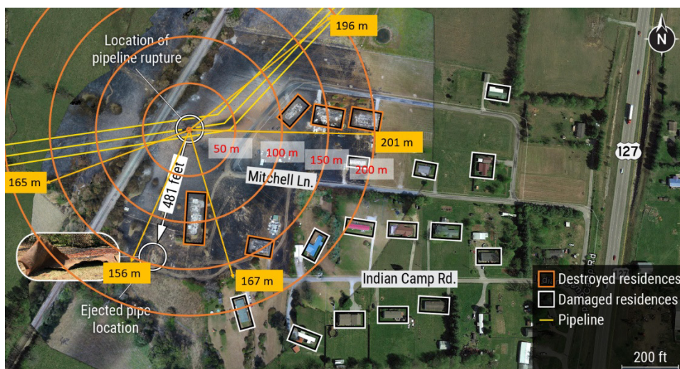
Figure 13 Damage after the pipeline rupture in Danville. Source: NTSB [34] with annotations by the authors.
