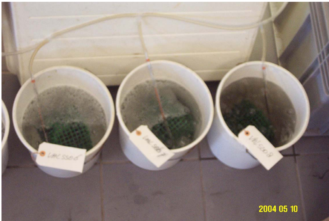
Picture 1 Mussel contamination experiment (faecal coliforms and Escherichia coli)
