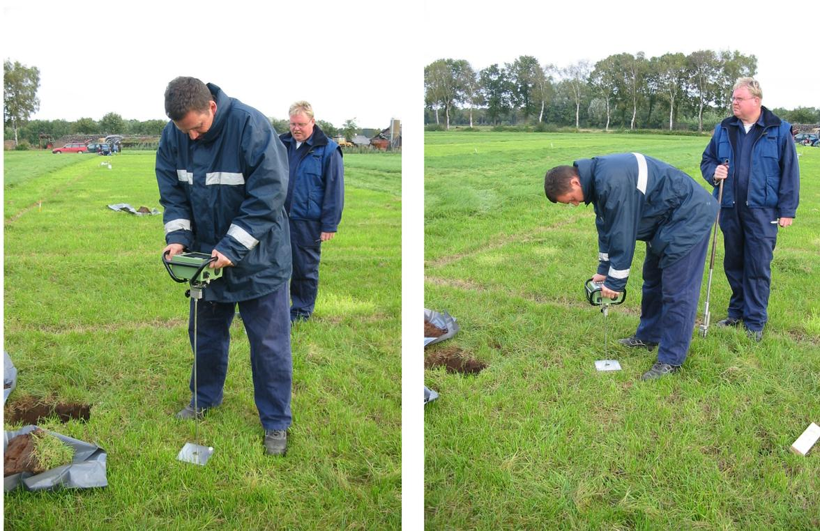
**Figure 8. Measuring penetration resistance in the field using a penetrometer. A cone (top angle 60°) with a surface area of 1 cm<sup>2</sup> is placed at the end of the rod (about 1 m long). The rod is pushed into the soil with a speed of about 2 cm/s. Speed and depth are measured using a sensor that sends a signal to the reflector plate resting on the soil surface.**
