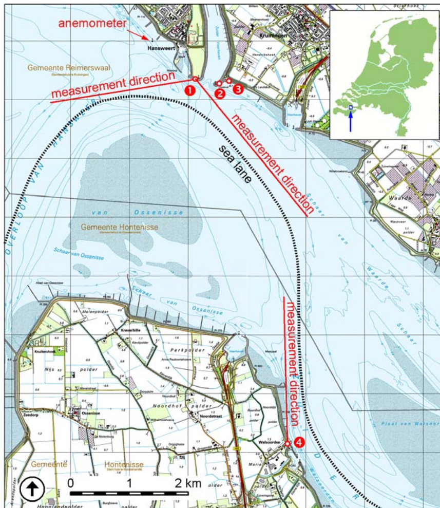
Figure 2-4. The measurement locations at Hansweert and Walsoorden. The locations at Hansweert are marked with ①, ② and ③, and the measurement location at Walsoorden is marked with ④. For locations 1 and 4, the measurement directions are shown. Anemometer: measurement mast of Rijkswaterstaat where wind speed, wind direction and water level are measured.
