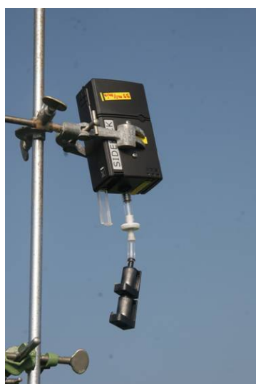
Photograph 2 Pump with dust filter and two ThermoSorb-N cartridges
