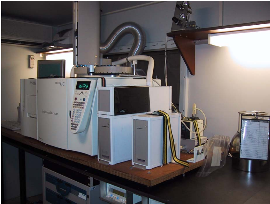
Foto 1: Interieur mobiel laboratorium ML2, GC-MS Trace 2000 Thermo Finnigan
