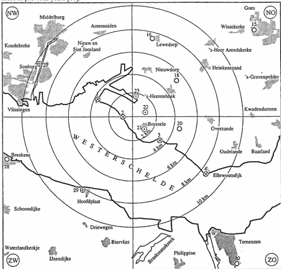
Figure 9.1: Overview of monitoring locations for the monitoring program in the vicinity of the nuclear power plant at Borssele as conducted by NRG. The numbers given in Table 9.1 correspond with the locations in the map.
