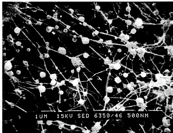
Fig.4. Scanning electron microscopic photographs of ultrafine (A) and fine (B) ammonium bisulfate particles. Ultrafine particles were collected on a VMTP filter (pore size= 50 nm) and fine particles on a VALP Teflon filter (pore size 1 \mu\text{m} ). Both pictures show a white line that can be used to calculate the magnification and thus the diameter of the particles.
