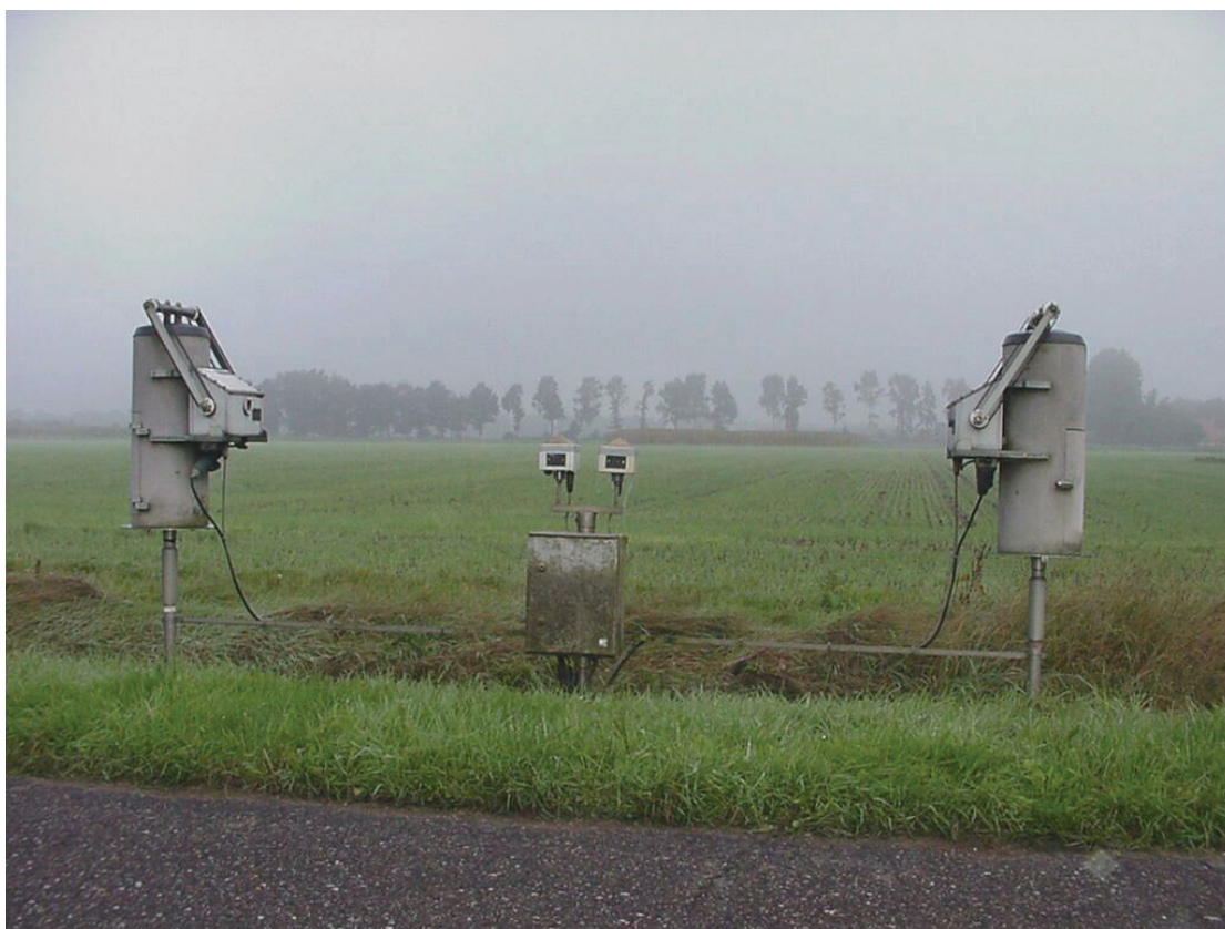
Figure 3: Example of wet-only samplers with rain sensor in the middle at Vredepeel (location 131).
