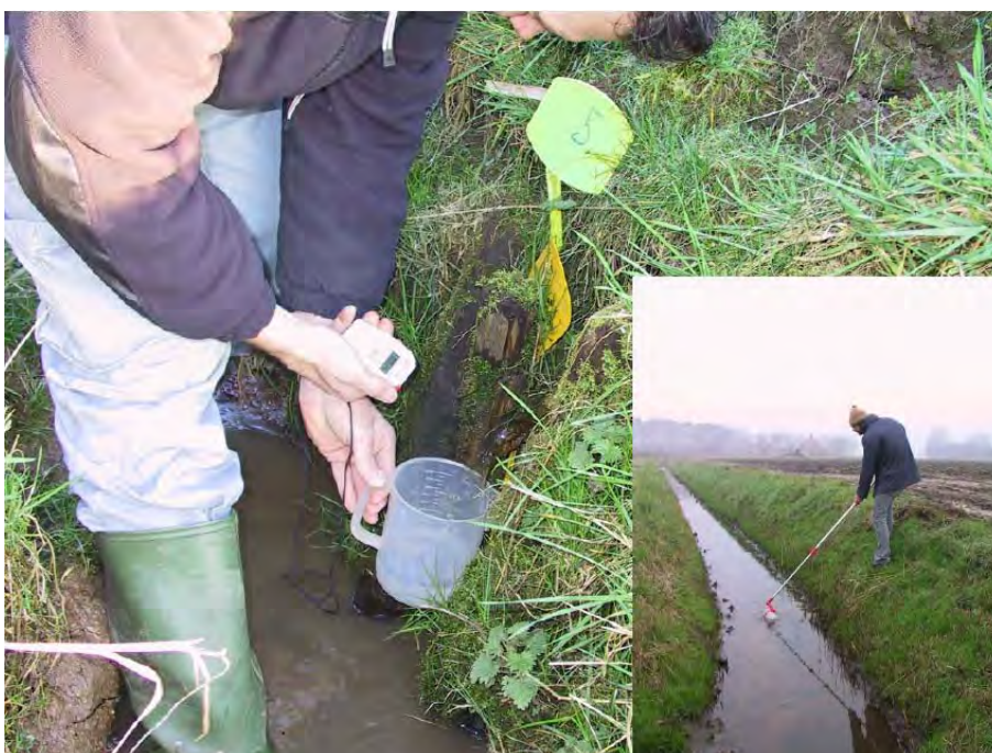
Figure 12 Sampling of tile-drain water (left) and ditch water (right) in the clay region.
