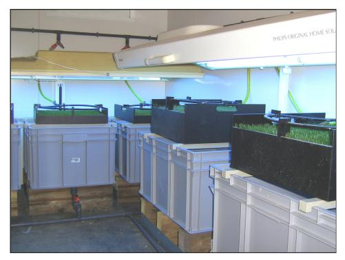
Figure 5.2 Setup of the artificial turf test system. Artificial turf is exposed to UV-radiation, ozone, a temperature cycle from -5 to 40 °C and rainfall. Leachate is collected in the grey containers (taken from Hofstra, 2008).
