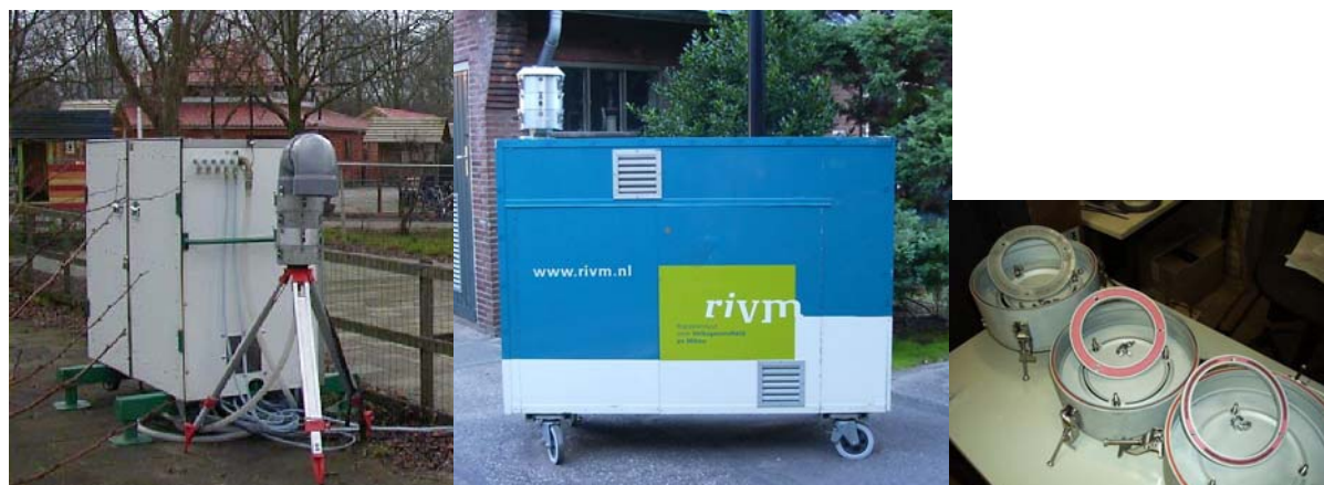
Figure 2.1 HEPMEAP PM collection device with the HVCI next or on top of a box with the pump to pull the air through the impactor (left two panels) and the inside of the HVCI showing the pink PUF with collected PM (black) of the fine mode stage (right panel).
