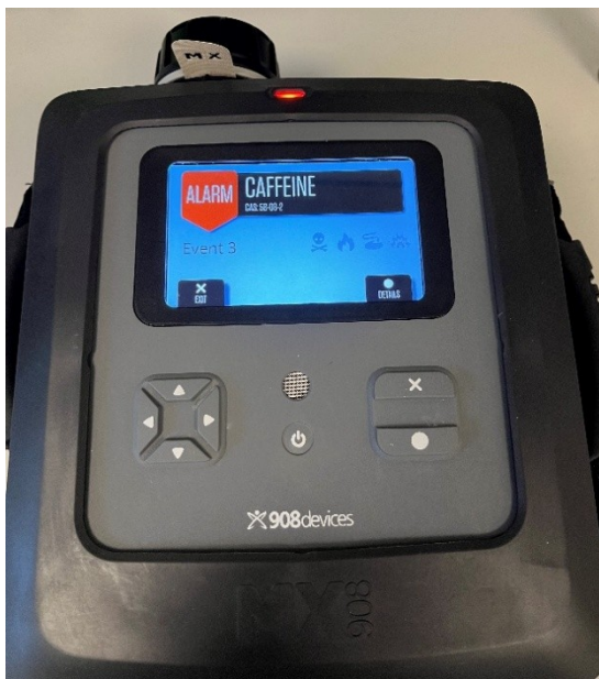
Photo 4: caffeine positive test result displayed by the MX908 device
