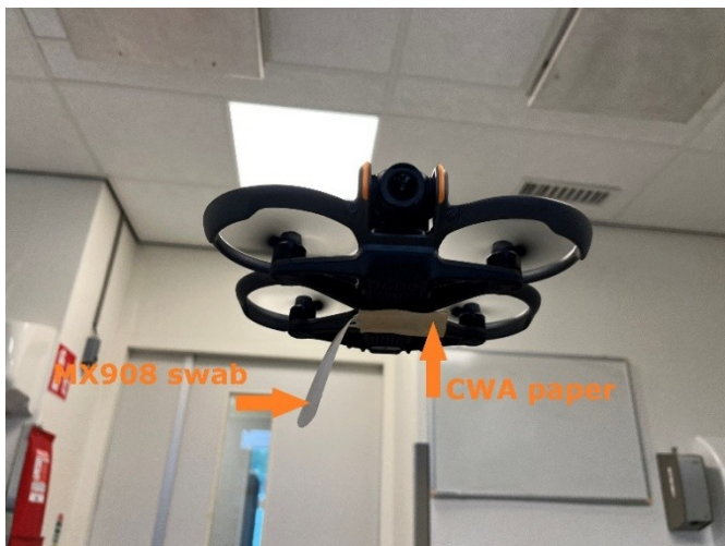
Photo 1: DJI Avata 2 UAV equipped with MX908-swab and CWA detection paper
