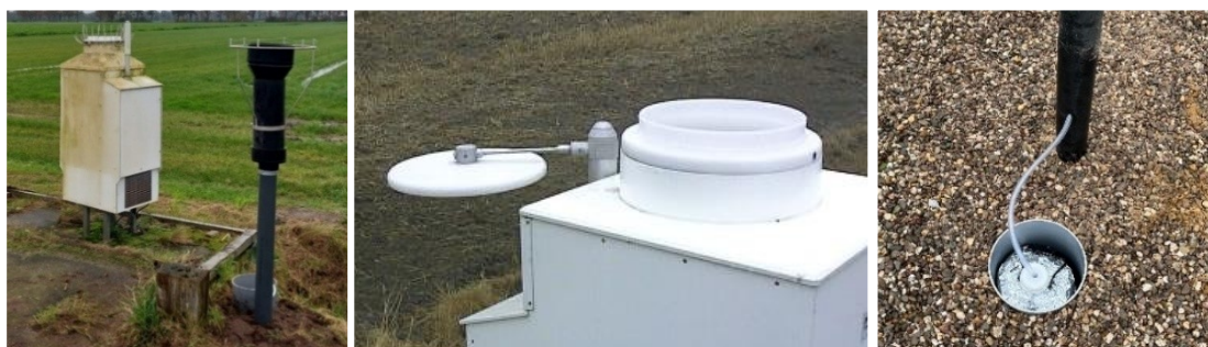
Left photo: The wet-only (white) and bulk collector (black) at Vredepeel. Center photo: The wet-only collector with the lid is open. Right photo: and the bulk collector's bottle in the ground.
