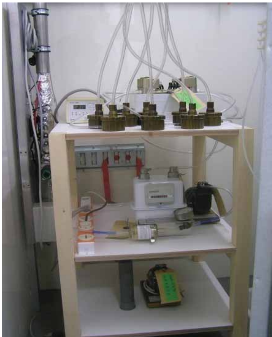
Figure 1.1 The Low Volume Sampler as applied in NAQMN (LVS-RIVM)
