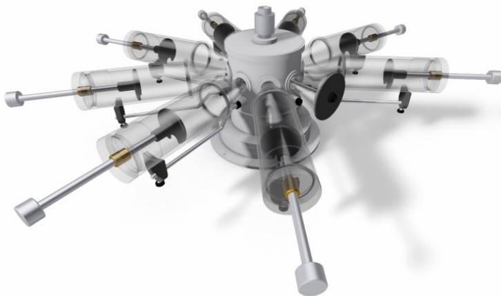
Figure 29. Drawing of an inhalation tower equipped with 8 tubes and 1 sampling probe.
