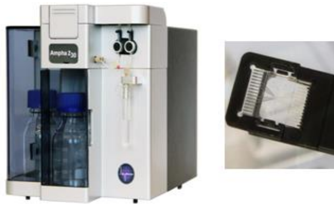
Figure 1: Impedance flow cytometer Ampha Z30 (left) and microfluidic chip (right).
