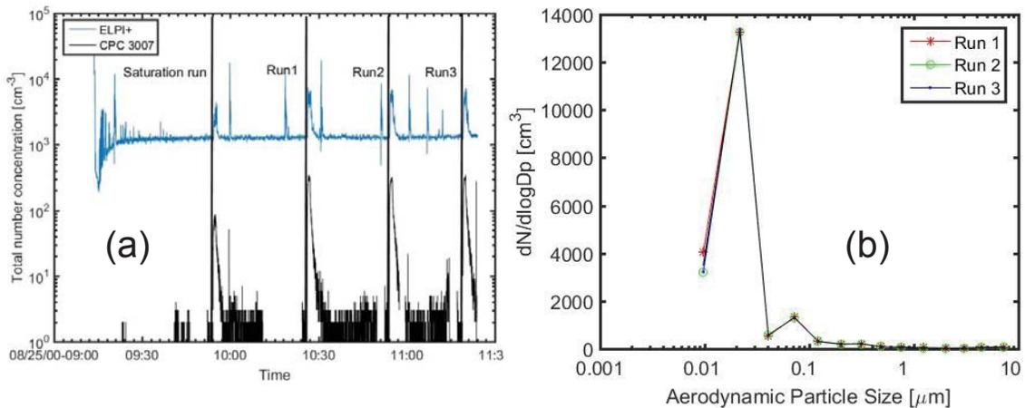
Figure 28: Time profile of the number concentration (a) and number-weighted size distribution versus aerodynamic equivalent diameter (b) obtained with the MWCNT 400.
