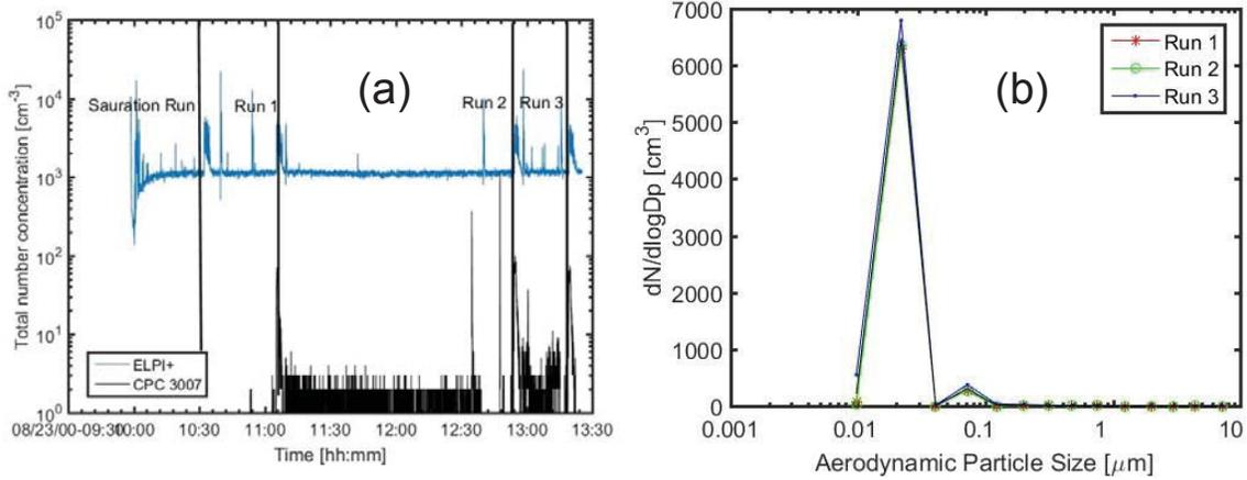
Figure 27: Time profile of the number concentration (a) and number-weighted size distribution versus aerodynamic equivalent diameter (b) obtained with the MWCNT 401.
