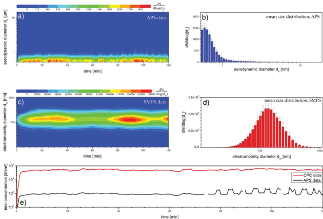
Figure 10: a) Histogram of the particle size distribution measured with the APS; b) Measured mean size distribution over the course of the dustiness test. Accordingly; c) and d) Histograms of the particle size distribution measured with the SMPS and the mean size distribution, respectively; e) Total particle number concentration, measured with the APS and the SMPS as a function of time.
