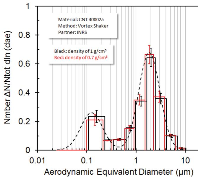
Figure 20: Number-weighted size distribution versus aerodynamic equivalent diameter time-integrated over the period of vibration (60 s) for the CNT 40002a. Histogram is presented for two densities (1 and 0.7 g/cm<sup>3</sup>); average values are shown with their standard deviation over 3 experiments. Dotted line corresponds to the fitted distribution obtained for the density of 1 g/cm<sup>3</sup>.
