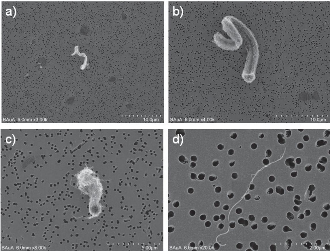
Figure 33: SEM images of NM 400 particles collected on nuclear pore filter samples (0.1 L/min, 20 Hz, 4 V).
