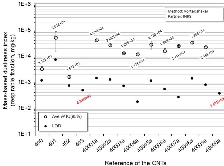
Figure 14: Respirable mass dustiness index (in mg/kg) for the 14 CNTs tested at INRS. Average values (empty circles) are presented with their 95% confidence interval. Black circles correspond to the LOD.
