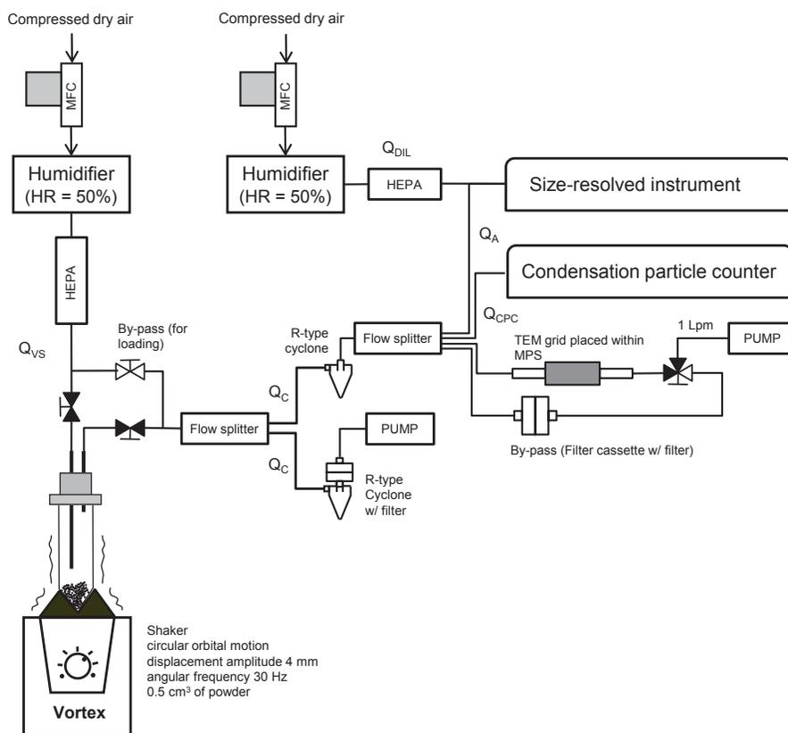
Figure 1: Experimental set-up of the vortex shaker method for determining the number and mass based dustiness index, for characterizing particle-size distribution of the emitted aerosol, and for collecting airborne particles for subsequent EM observations.
