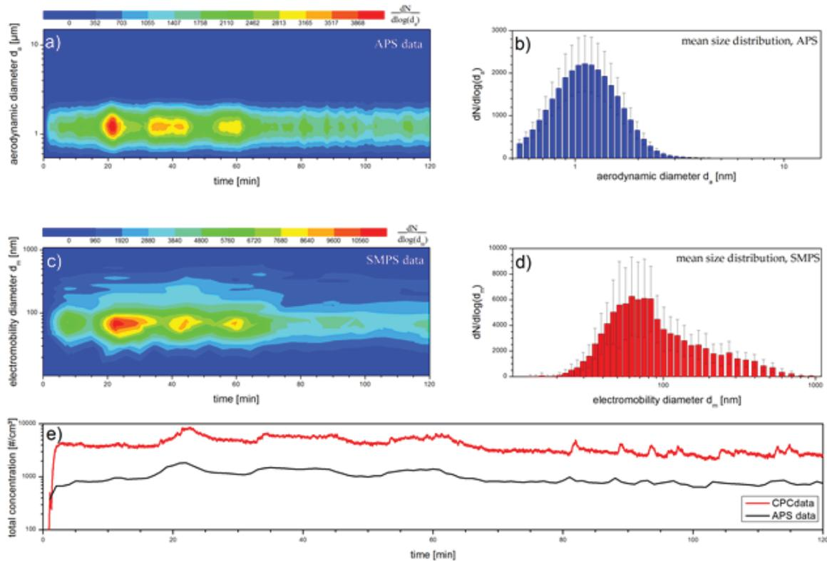
Figure 31: Dustiness profile of the tangled bed of NM 400. (a) APS particle size distribution as a function of time. (b) APS mean particle size distribution. (c) SMPS particle size distribution as a function of time. (d) SMPS mean particle size distribution. (e) CPC particle number concentration as a function of time.
