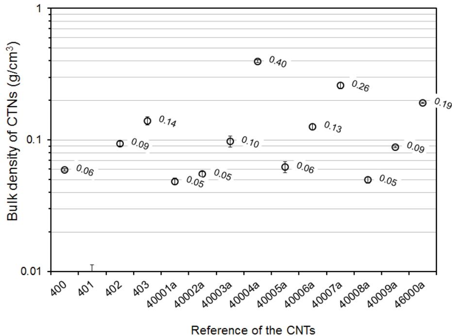
Figure 13: Bulk density of the 14 CNTs tested at INRS. Average data are shown with their 95% confidence intervals.
