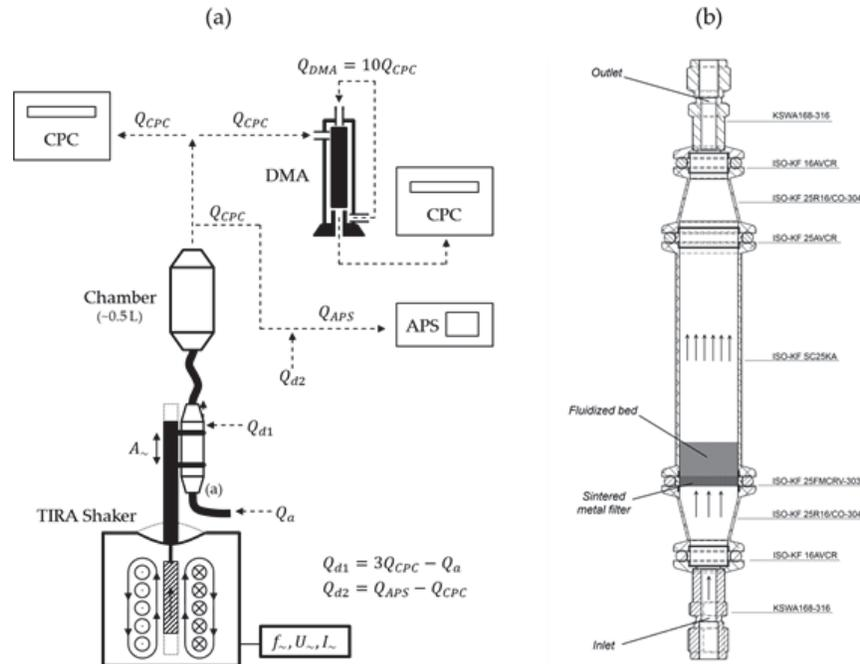
Figure 9: (a) Experimental setup and flow scheme of the dustiness test. Detailed descriptions of both figures are given in the text. (b) Schematic layout of the container that retains the fluidized bed.
