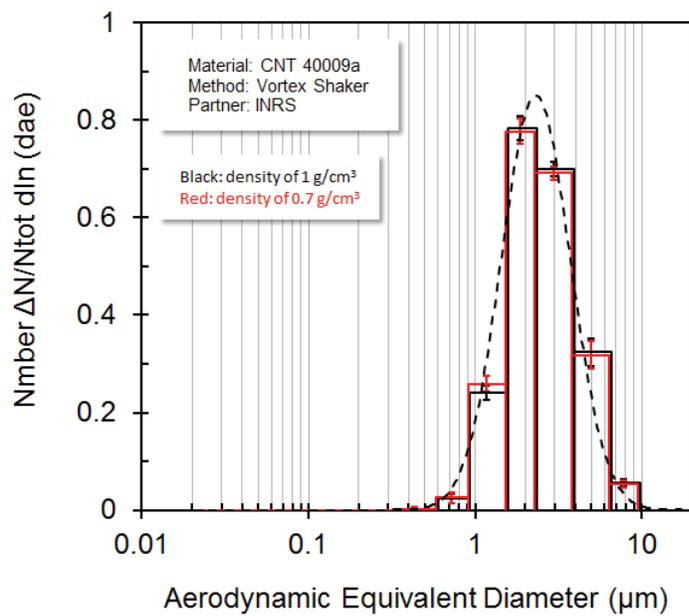
Figure 21: Number-weighted size distribution versus aerodynamic equivalent diameter time-integrated over the period of vibration (60 s) for the CNT 40009a. Histogram is presented for two densities (1 and 0.7 g/cm<sup>3</sup>); average values are shown with their standard deviation over 3 experiments. Dotted line corresponds to the fitted distribution obtained for the density of 1 g/cm<sup>3</sup>.
