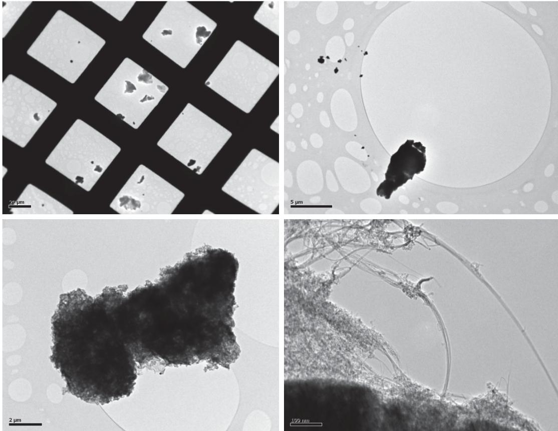
Figure 22: TEM images of airborne CNT sampled during the SWCNT 46000a Vortex Shaker experiments. Sampling duration of 10 s with the MPS equipped with 400 mesh Holey Carbon Film TEM grids. Images made by LEPI for INRS.
