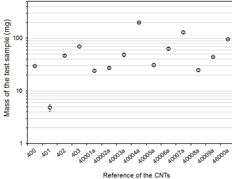
Figure 12: Average masses used for dustiness testing for each of the 14 CNTs tested with the vortex shaker method. Average values are presented with their standard deviation.
