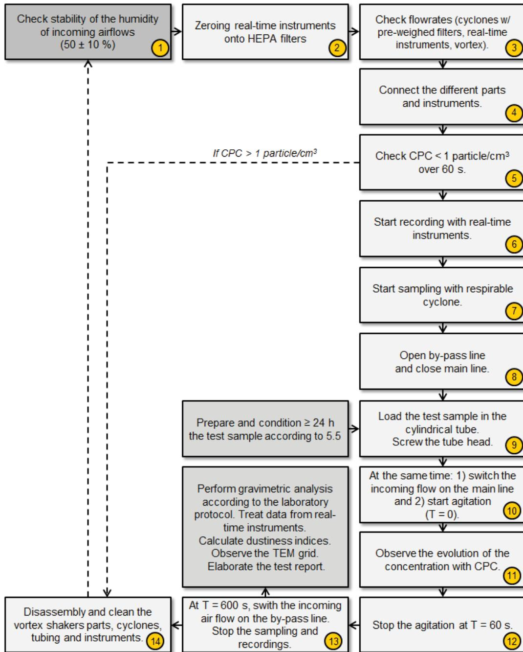
Figure 4: Flow diagram describing the different stages of the test protocol used by INRS.
