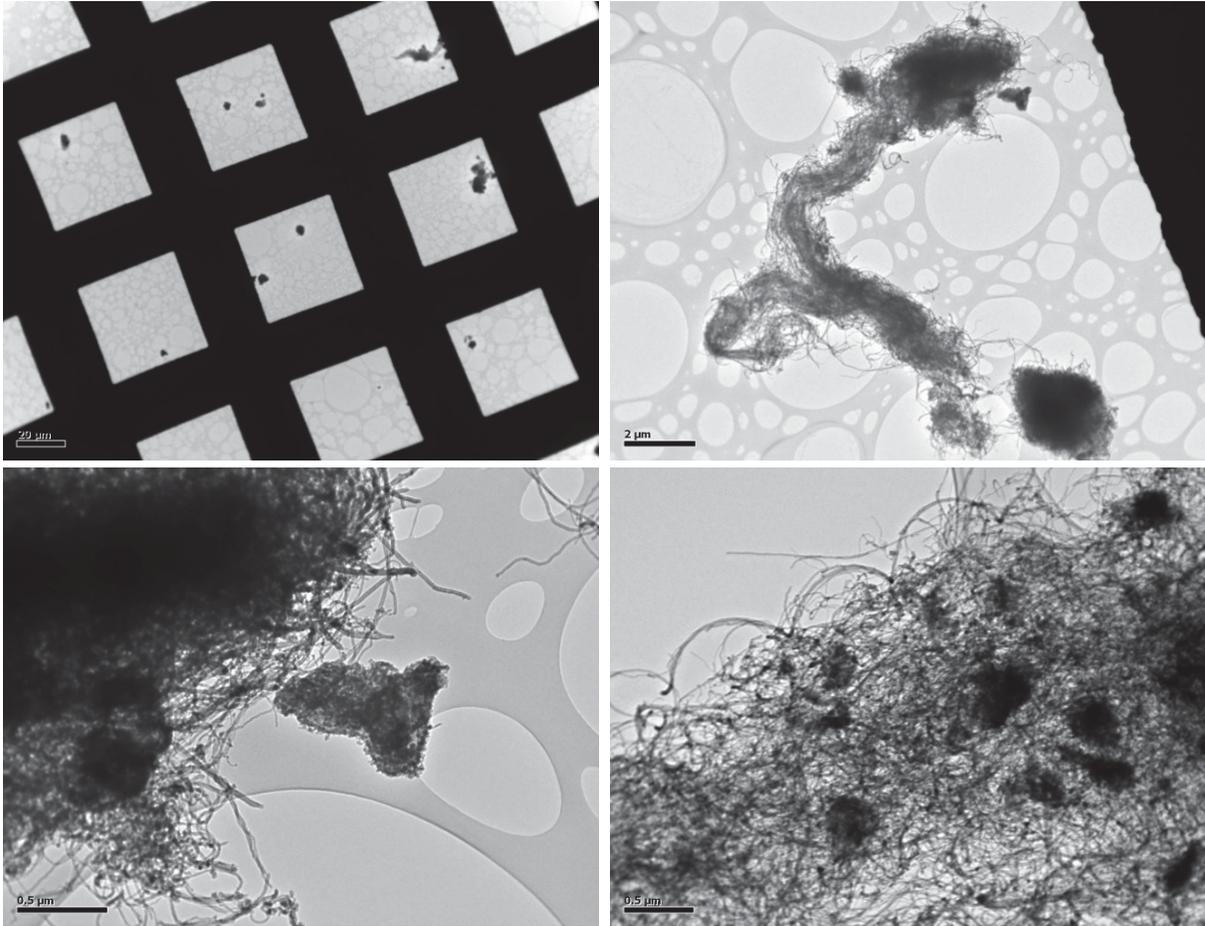
Figure 24: TEM images of airborne CNT sampled during the MWCNT 40002a Vortex Shaker experiments. Sampling duration of 10 s with the MPS equipped with 400 mesh Holey Carbon Film TEM grids. Images made by LEPI for INRS.
