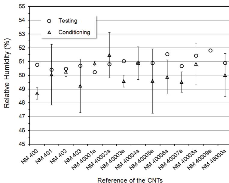
Figure 11: Relative humidity (in %) during the conditioning of the test samples (> 24 h) and during the dustiness testing (600 s) for the nanotubes. The average values for the conditioning are shown their standard deviations.
