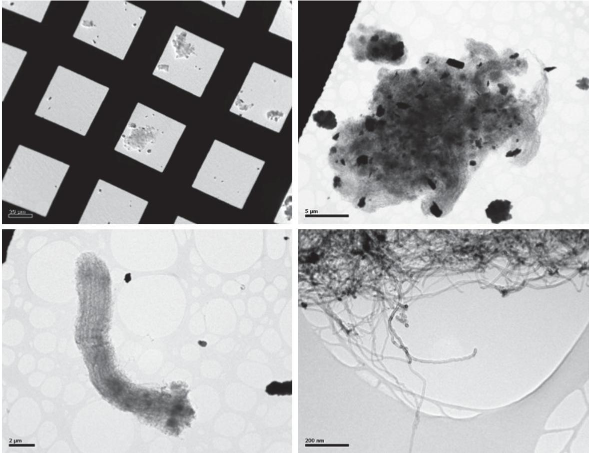
Figure 25: TEM images of airborne CNT sampled during the MWCNT 400 Vortex Shaker experiments. Sampling duration of 10 s with the MPS equipped with 400 mesh Holey Carbon Film TEM grids. Images made by LEPI for INRS.
