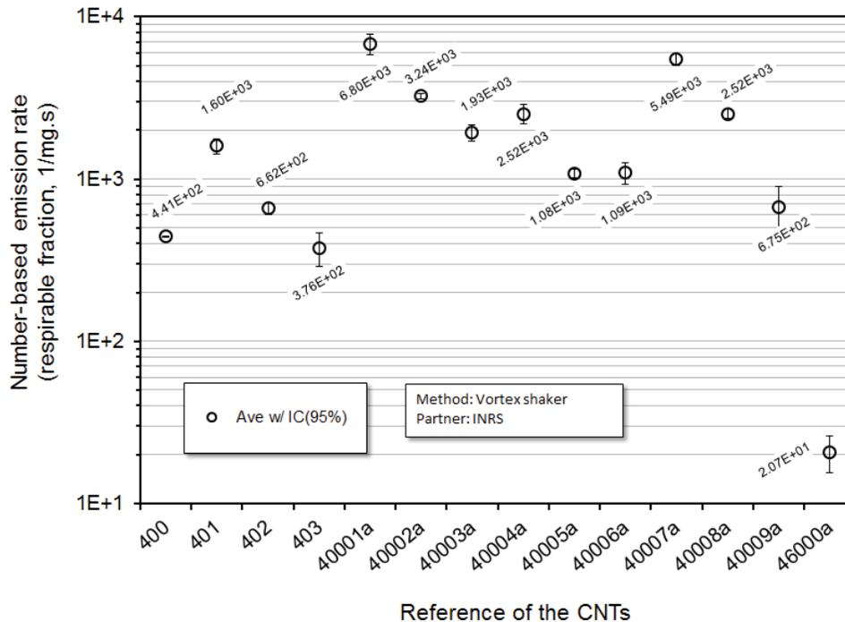
Figure 16: Number-based emission rate (1/mg.s) in respirable fraction over the vibration period (60 s) for the 14 CNTs tested at INRS. Average values (empty circles) obtained on three repeats are presented with their 95% confidence interval.
