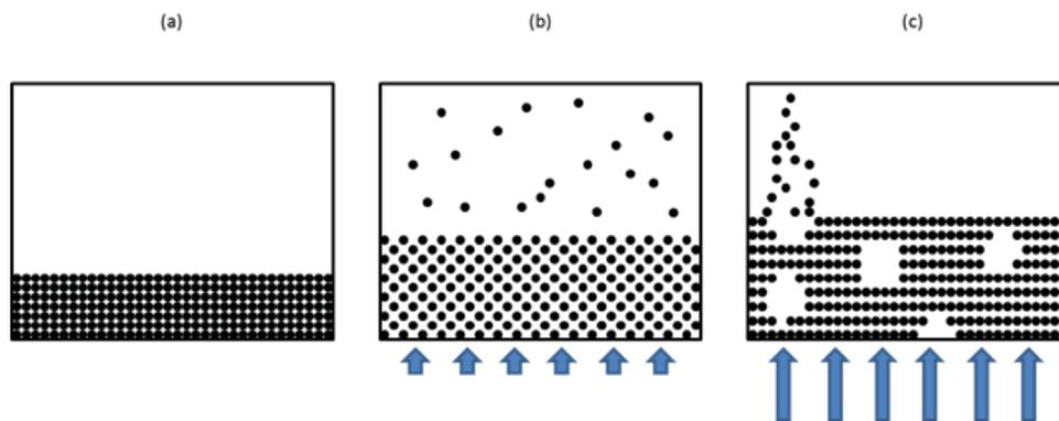
Figure 8: Different states of a powder bed during fluidization: (a) fixed bed – no flow, (b) incipient bed - flow near minimal fluidization velocity, (c) bubbling bed – high flow.
