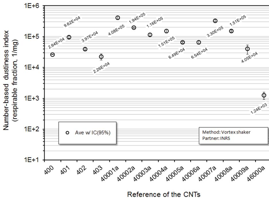
Figure 15: Respirable number dustiness index (in 1/mg) for the 14 CNTs tested at INRS. Average values (empty circles) are presented with their 95% confidence interval
