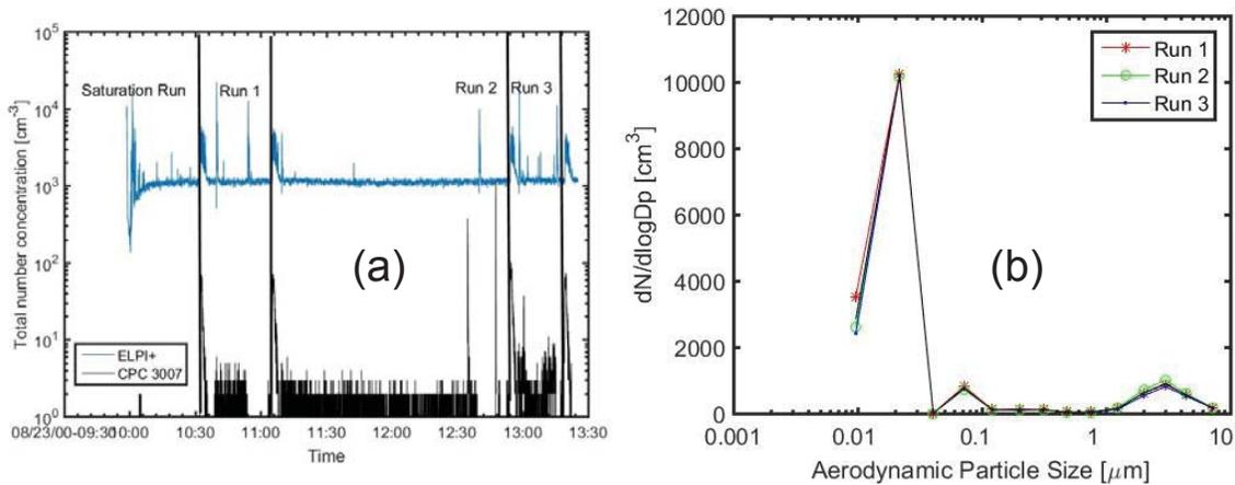
Figure 29: Time profile of the number concentration (a) and number-weighted size distribution versus aerodynamic equivalent diameter (b) obtained with the SWCNT 46000a.
