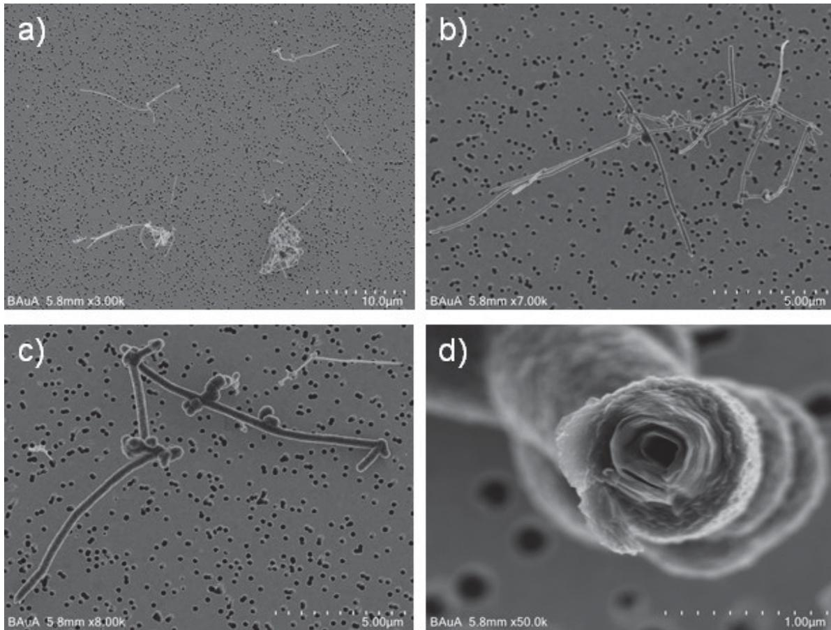
Figure 35: SEM images of NM 401 particles on nuclepore filter samples (0.1 L/min, 20 Hz, 4V).
