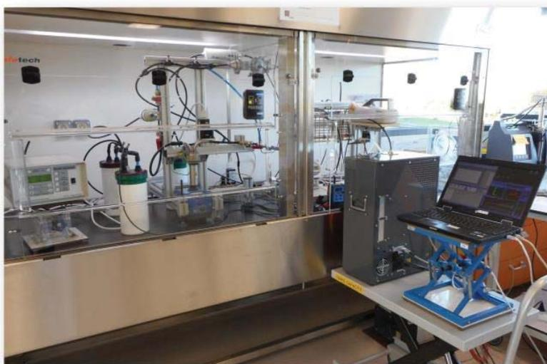
Figure 3: Full view of the vortex shaker test bench positioned in specially designed ventilated enclosure.
