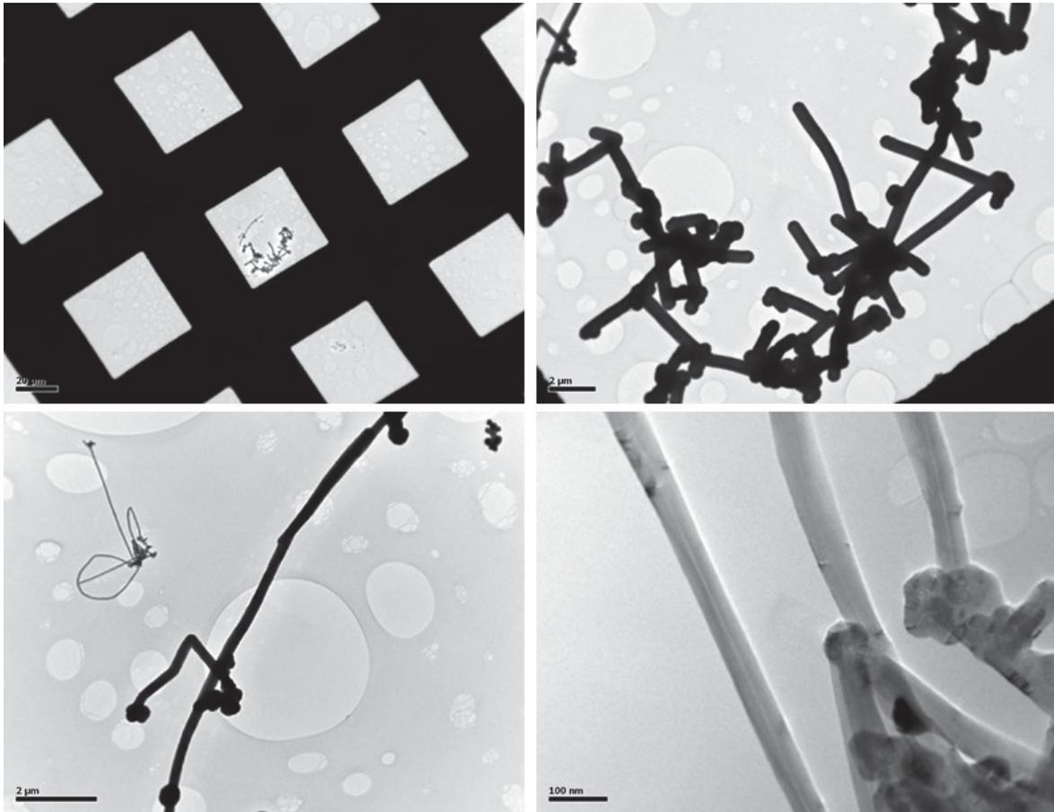
Figure 26: TEM images of airborne CNT sampled during the MWCNT 401 Vortex Shaker experiments. Sampling duration of 10 s with the MPS equipped with 400 mesh Holey Carbon Film TEM grids. Images made by LEPI for INRS.
