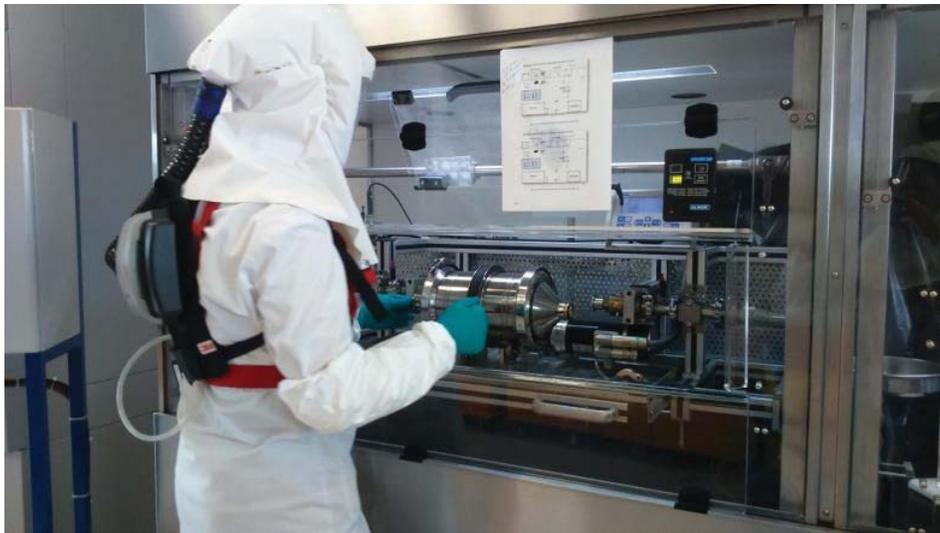
Figure 6: Personal equipment used by the operator while cleaning a test bench after a dustiness test.
