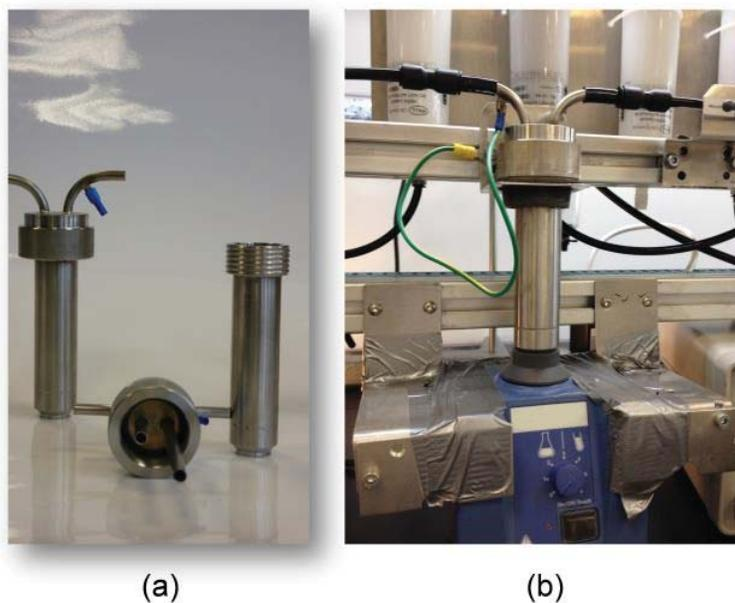
Figure 2: View of two stainless steel cylindrical tubes (a) and one positioned in test bench on the vortex shaker (b).
