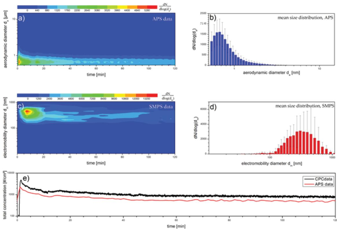
Figure 34: Dustiness profile of the tangled bed of NM 401. (a) APS particle size distribution as a function of time. (b) APS mean particle size distribution. (c) SMPS particle size distribution as a function of time. (d) SMPS mean particle size distribution. (e) CPC particle number concentration as a function of time.
