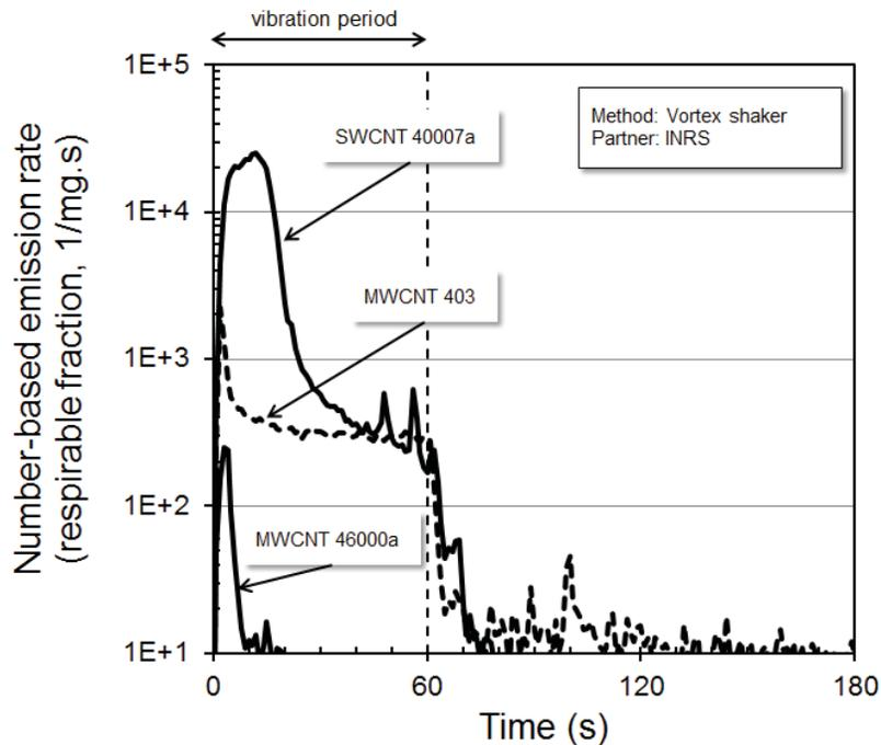
Figure 18: Number-based emission rate (1/mg.s) in respirable fraction versus time for three of the tested CNT.
