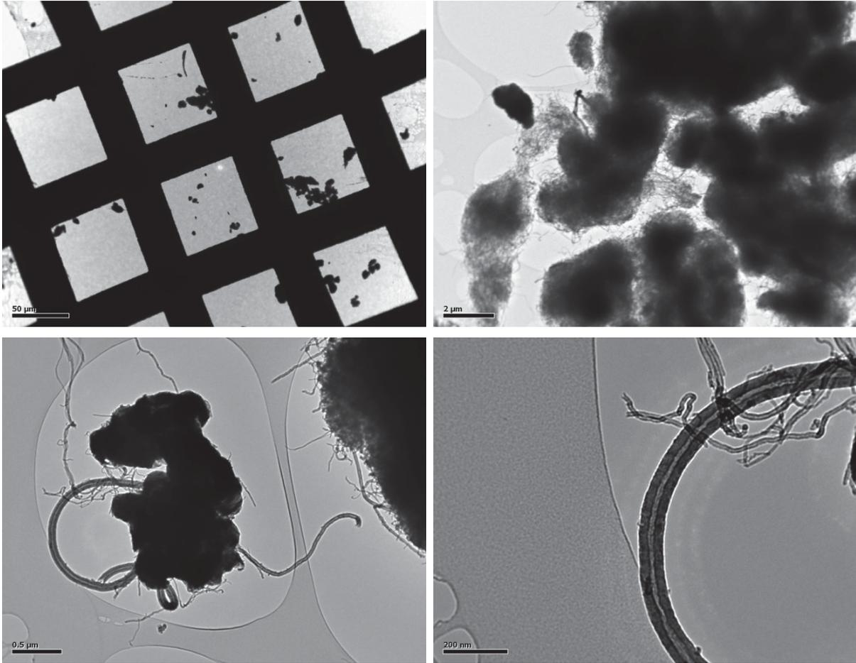
Figure 23: TEM images of airborne CNT sampled during the MWCNT 40001a Vortex Shaker experiments. Sampling duration of 10 s with the MPS equipped with 400 mesh Holey Carbon Film TEM grids. Images made by LEPI for INRS.
