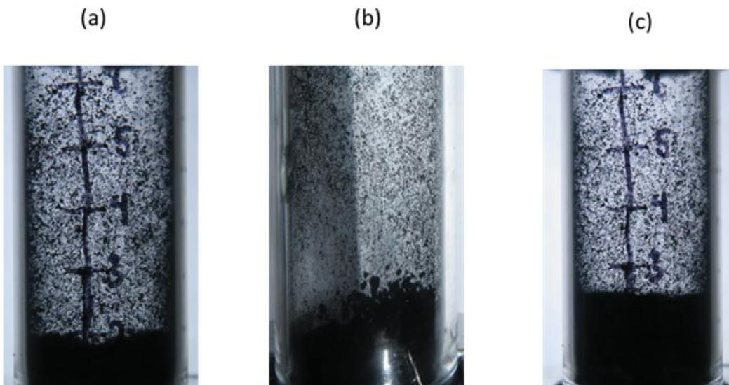
Figure 30: Different states of the powder bed during the VF-method: (a) Fixed bed, (b) Tangled bed, (c) Fluidized bed.
