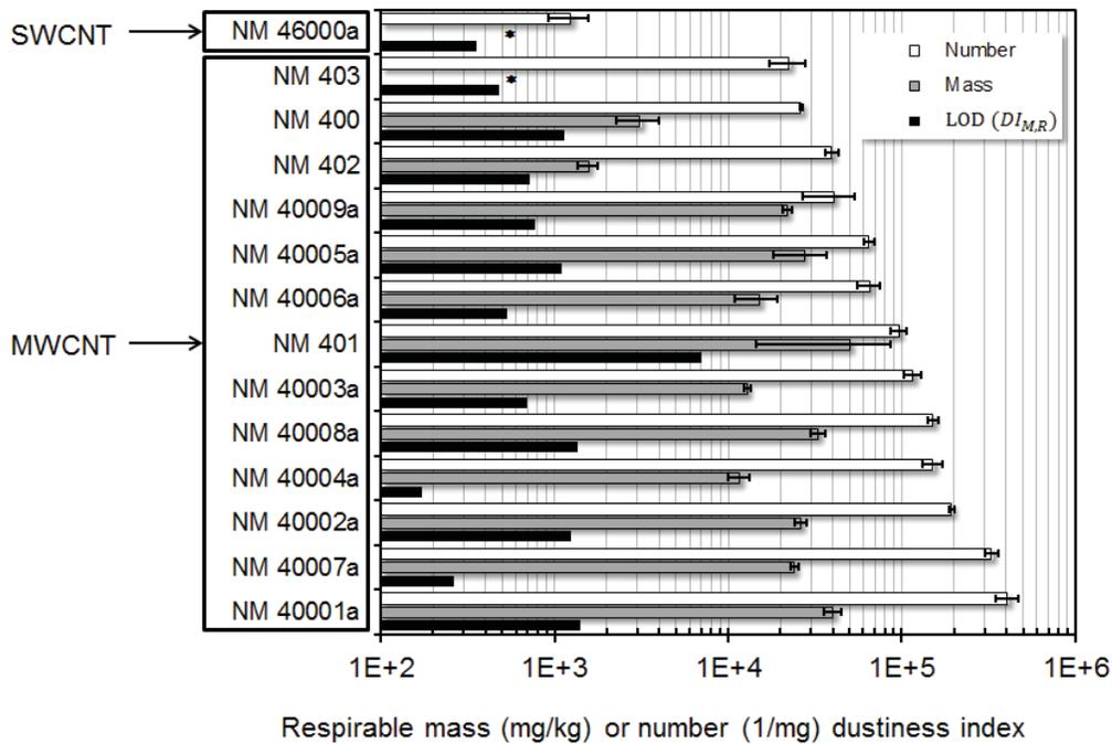
Figure 17: Respirable mass dustiness indices (in mg/kg) and respirable number dustiness indices (in 1/mg) for the fourteen CNTs obtained with the VS method. Average values are presented with their 95% confidence interval. Black bars correspond to the  $LOD(DI_{M,R})$ . Symbol \* indicates that the mass dustiness indices obtained were below the  $LOD(DI_{M,R})$ .
