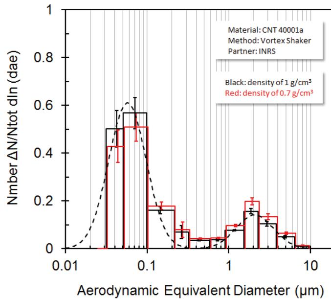
Figure 19: Number-weighted size distribution versus aerodynamic equivalent diameter time-integrated over the period of vibration (60 s) for the CNT 40001a. Histogram is presented for two densities (1 and 0.7 g/cm<sup>3</sup>); average values are shown with their standard deviation over 3 experiments. Dotted line corresponds to the fitted distribution obtained for the density of 1 g/cm<sup>3</sup>.
