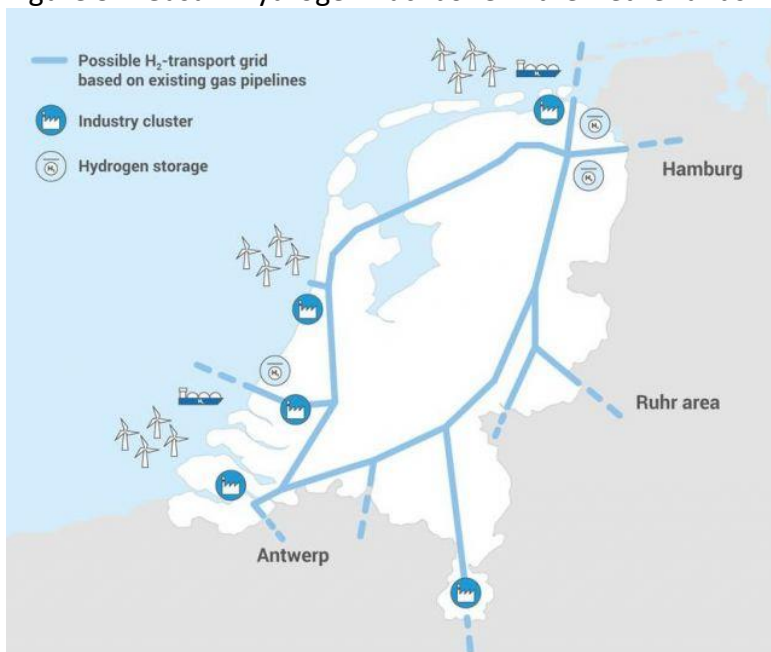
Figure 3.1 Gasuni hydrogen Backbone in the Netherlands
